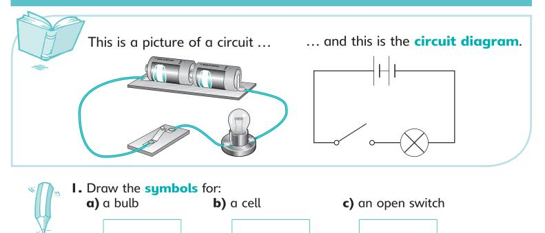
**2.** Draw circuit diagrams for these circuits. The first one has been started for you.
